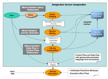
**Fig. 1.** Simplified Workflow – Mixed initiative design-time functionality supports users as they refine the specification of composite services, identify and select relevant services and compose them. Actual workflows often involve multiple iterations.
