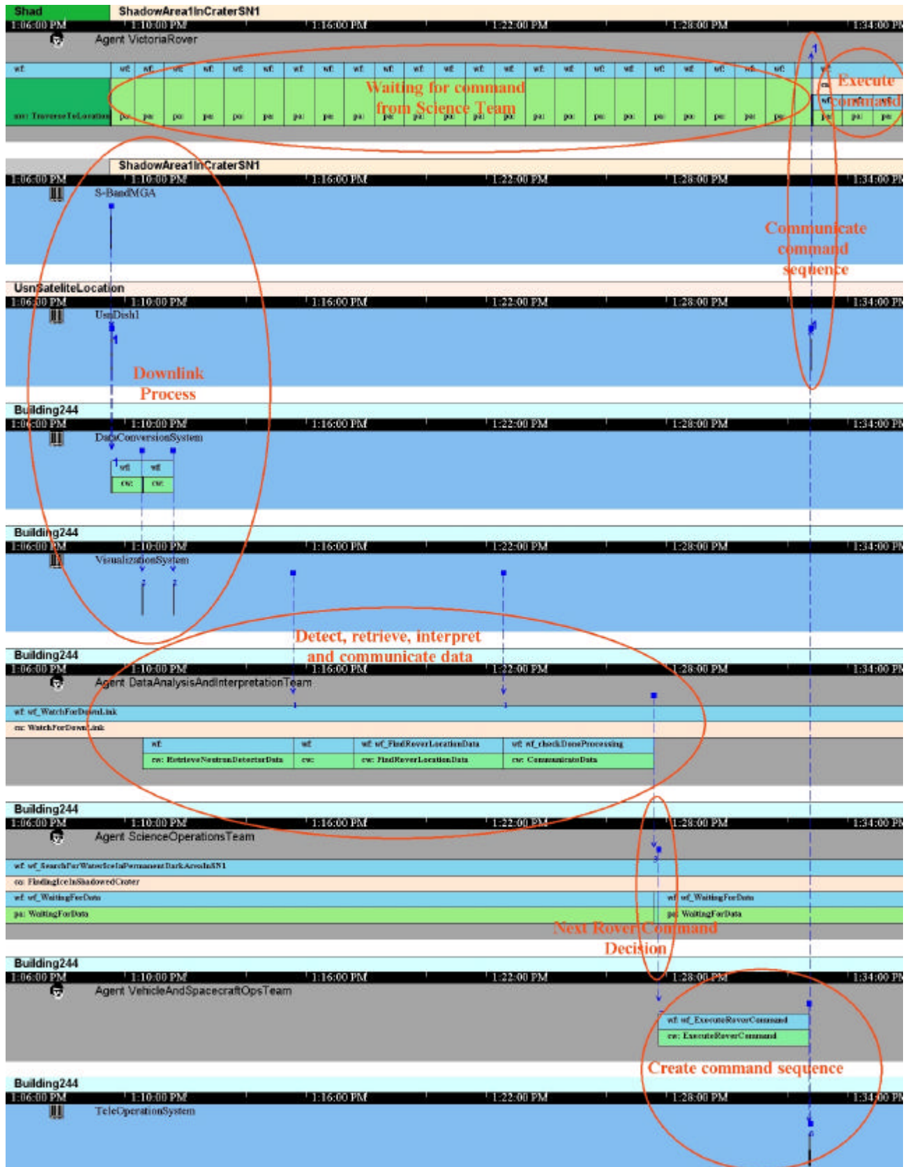
Figure 2. Simulation of downlink and second uplink command activities
